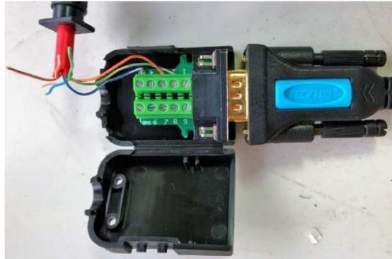
You can make up your own RJ-45 to conventional to RS-232 DB-9 female connecting cable using a standard Ethernet cable with the one end cut off. The standard color codes are:
